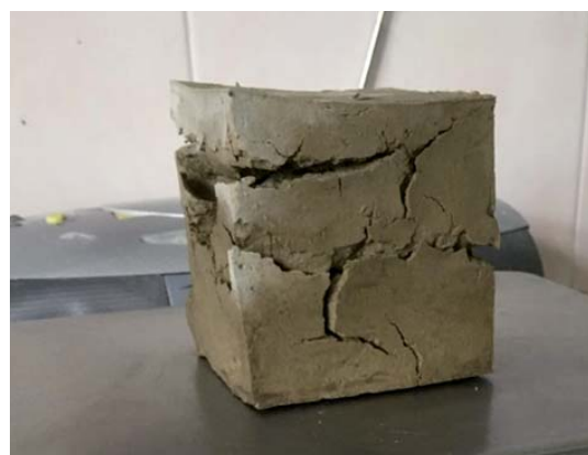
Rys. 1. Silne spękania próbki w wyniku skurczu suszenia Fig. 1. Strong cracks of the sample as a result of contraction of the drying
