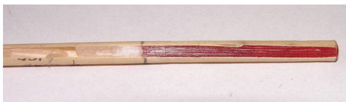
Fig. 1. Strengthened end of a test piece (chemo-hardening resin is visible inside destructed stem)
