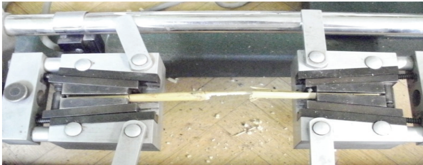
Fig. 2. Hounsfield’s extensometer with a failed test piece
