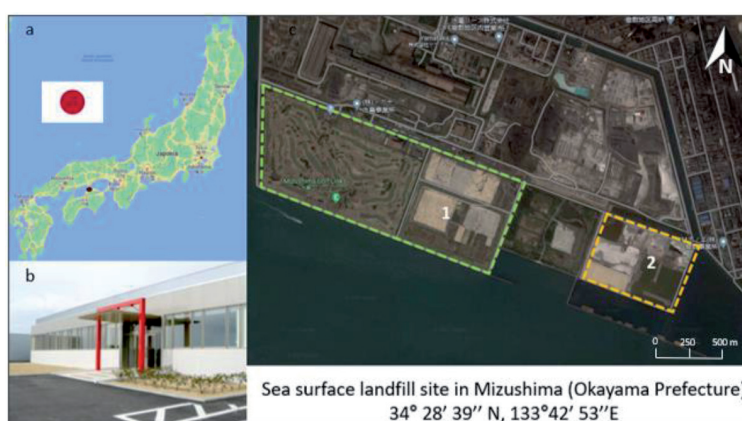
Fig. 3. Location of an industrial waste landfill in Mizushima: a – location of landfill on the map; b – recycling facilities; c – site plan of the landfill from above: (1) reclaimed old landfill and existing recycling facilities; (2) active part of the landfill
