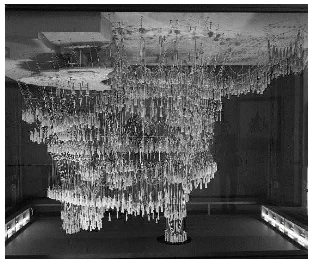
Fig. 4. Antoni Gaudi's spatial model – links adapt in shape to the load placed in the pouches (photo by A. Stefańska)
