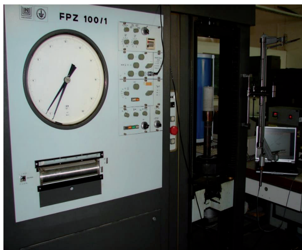
Fig. 5. Stands for testing the adhesion of steel to concrete
