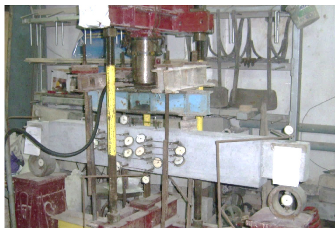
Fig. 6. General view of RC beam strengthened by RC jacket during test
