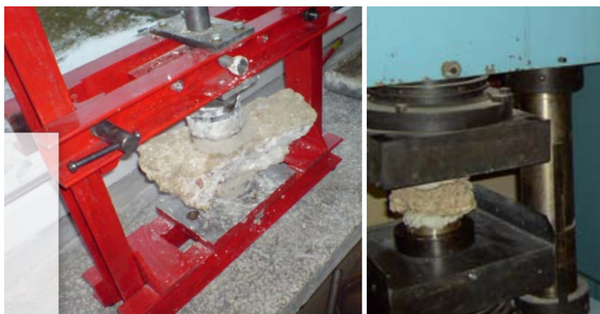
Fig. 5. Preparation for compression test of concrete irregular shape samples by concave punches and compression test of concrete by punches
