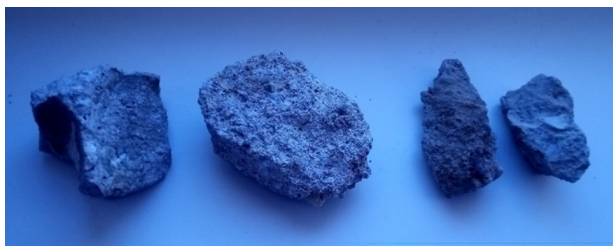
Fig. 3. Samples from concrete structures in Bražuolė hydroscheme
