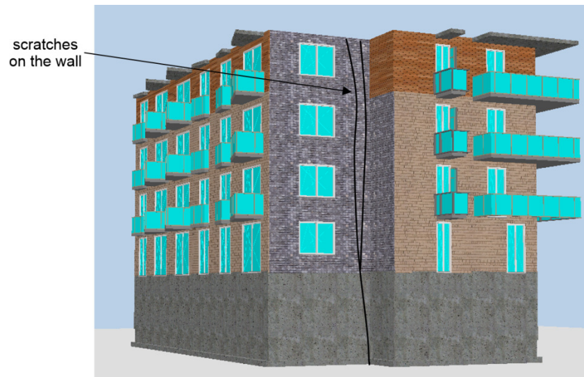
Fig. 6. Wall with scratches up to 1.4 mm wide
