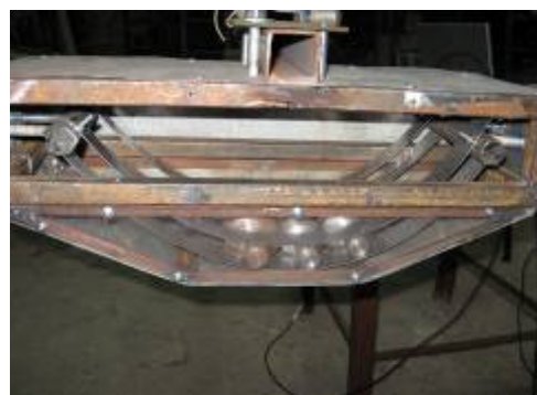
Fig. 6. The experimental example of DVA (in natural size)
