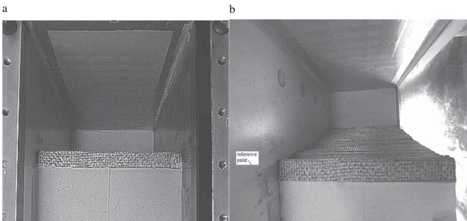
Fig. 5. View from above of model 1: a – before test number 1, b – after test number 1 with the reference point
