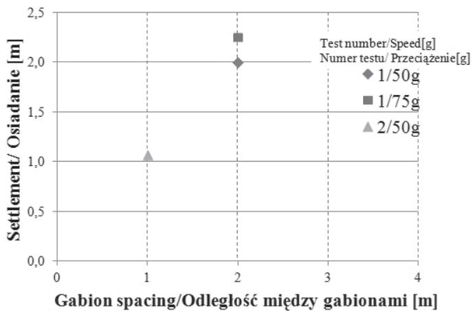
Fig. 7. Settlement vs gabion spacing
