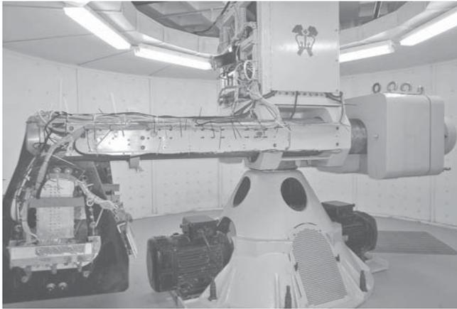
Fig. 1. Geotechnical centrifuge at Carleton Laboratory, Columbia University
