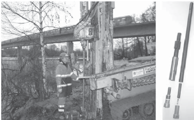
Rys. 11. System soil-rock total sounding CPTU [Nilsson i Löfroth 2012]
