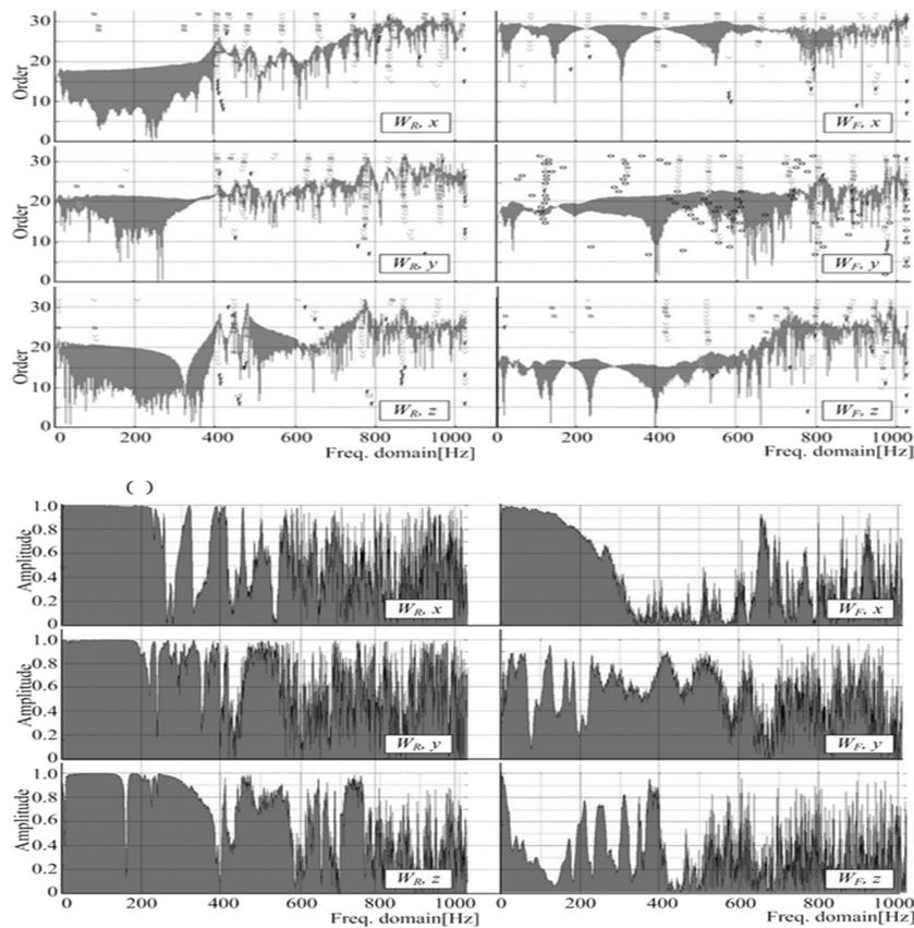
**Fig. 1.** Stabilization diagrams and coherence functions of recorded signals
