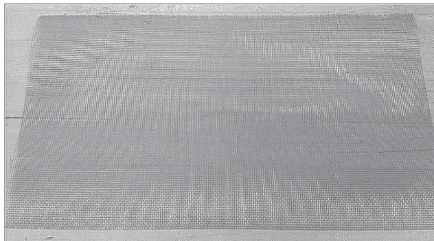
Fig. 4. Fiberglass Screen Reinforcement
