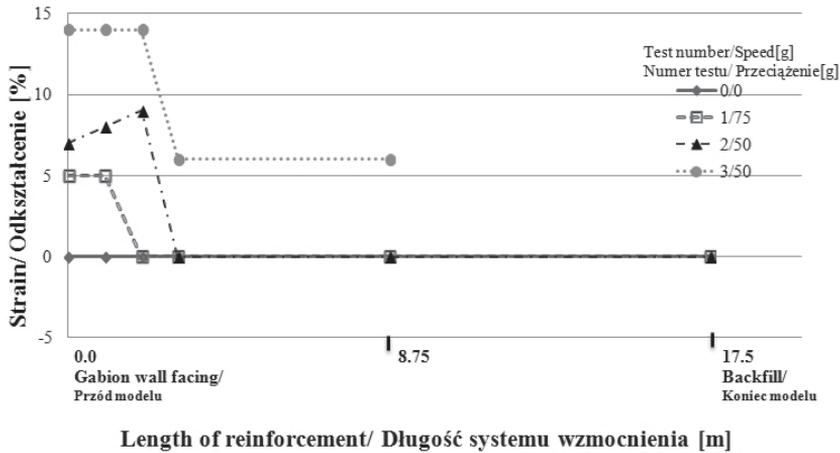
Fig. 6. Strain distributions in different point of reinforcement length under different centrifuge speed
